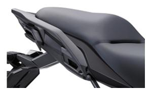
Larger grab handle provide a secure position for the pillion and double-up as the attachement point for the easy mount pannier system.
